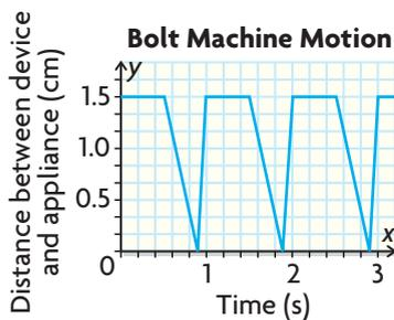
3. The motion of an automated device for attaching bolts to a household appliance on an assembly line can be modelled by the graph shown at the left.
