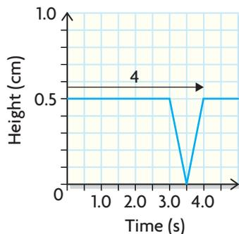
The cutting blade cuts a new section of metal strip every 4 s because the graph has a pattern that repeats every 4 s.
